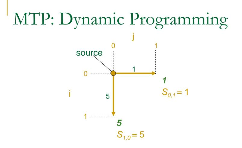
Calculate optimal path score for each vertex in the graph
